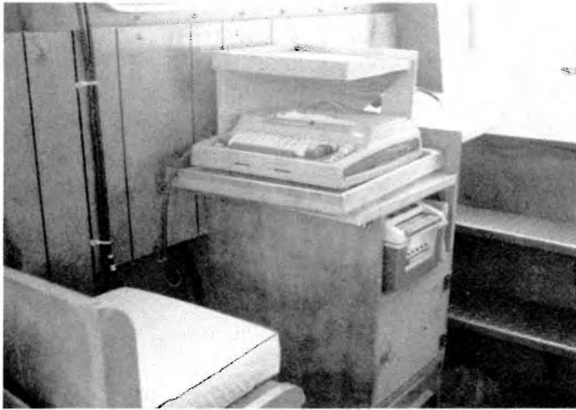
Figure 13. — Operator console and data tape recorder.
